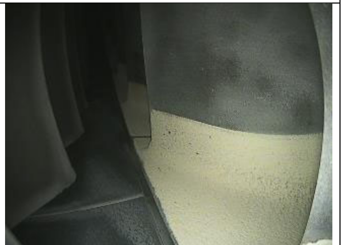
HPTN2 T/E and Outer Platform.
