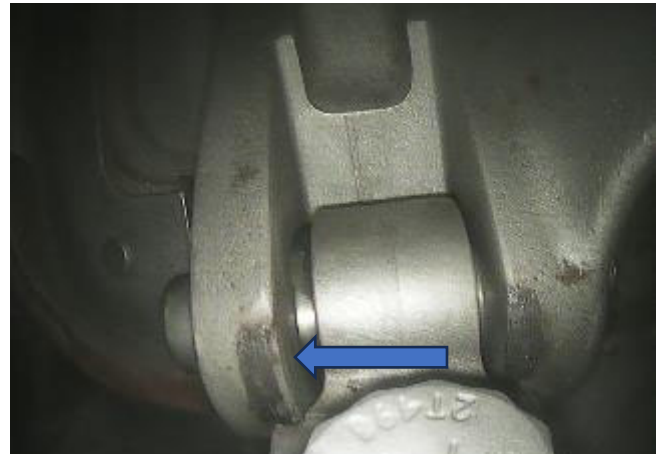
VBV Inspection / Hinge Contact Evident
